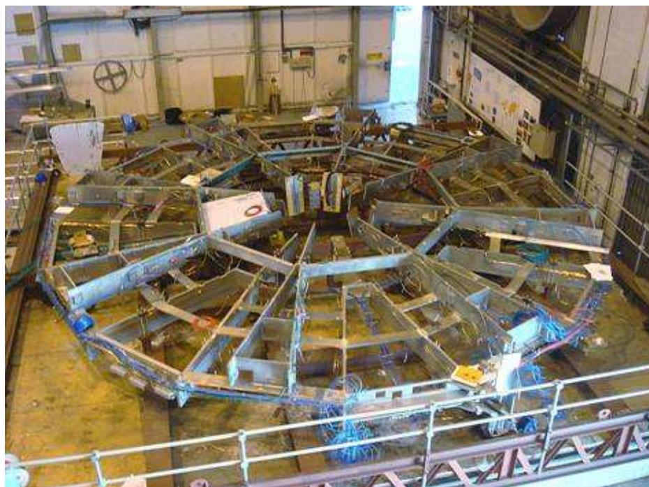
Fig. 4. One of the two Muon Small Wheels being assembled on the surface.
