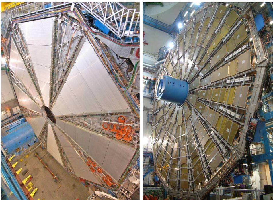
*Fig. 3. Completed Muon Big Wheels. Left: Precision MDT chambers. Right: trigger (TGC) chambers.*
