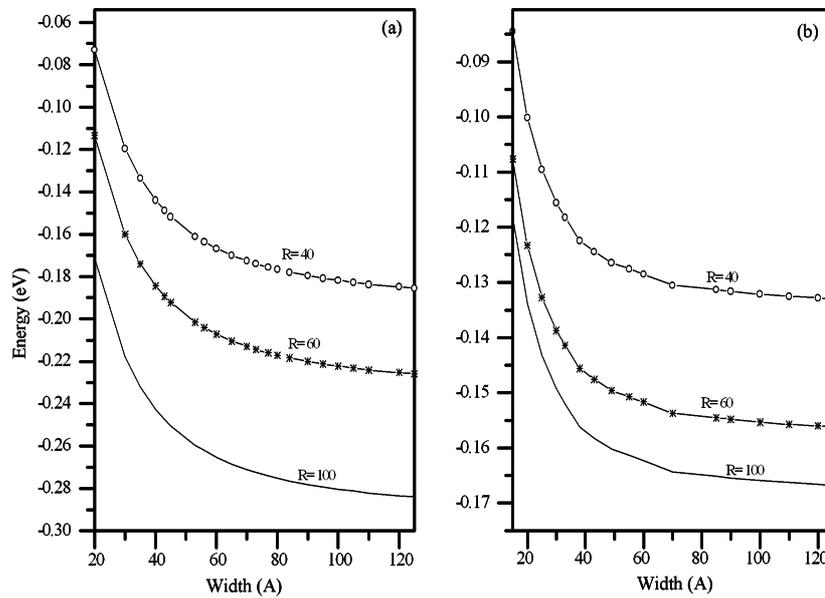
Fig. 4. (a) The electron ground-state energy as a function of the disc width  $L/2$  for three values of radius  $R = 40, 60$  and  $100$  Å. (b) The hole ground-state energy for the same three values of  $R$ .
