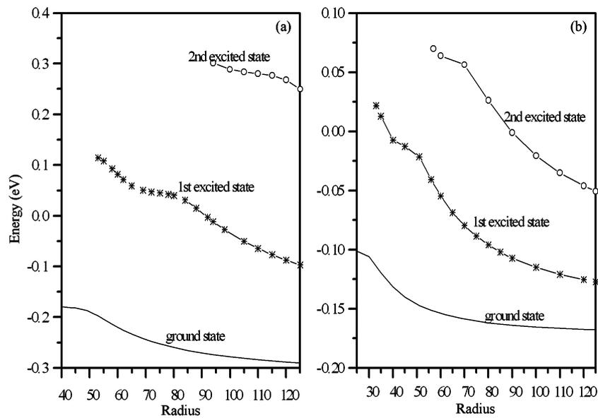
Fig. 5. (a) The electron ground and the first two excited states as a function of  $R$  for  $L/2 = 90$  Å and  $V = 0.3242$  eV. (b) The hole ground and the first two excited states for the same values of  $L/2$  and  $V = 0.1746$  eV.
