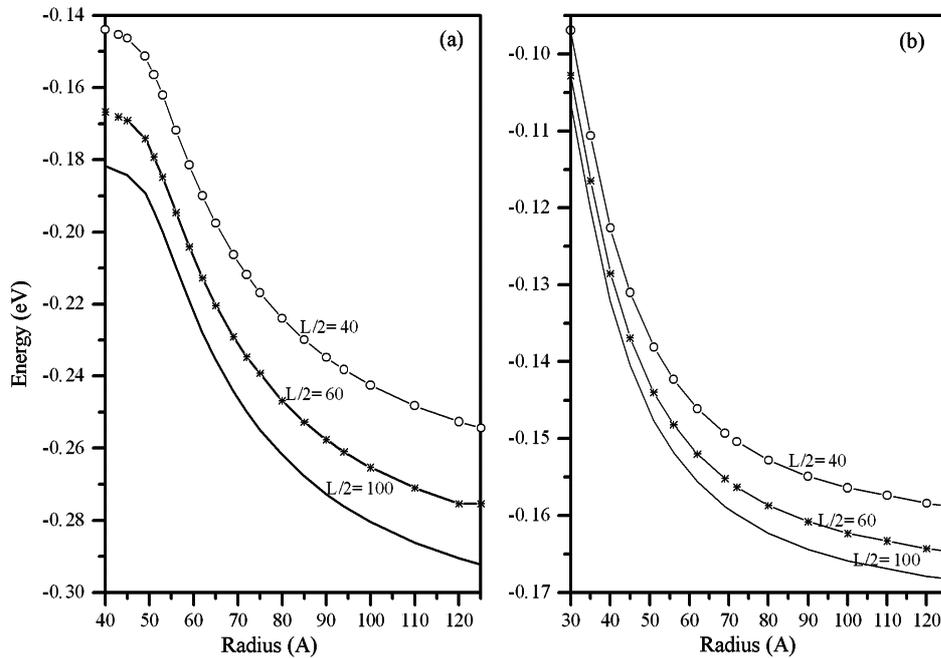
Fig. 2. (a) The electron ground-state energy (eV) vs. disc radius  $R$  for three values of disc width,  $L/2 = 40, 60$  and  $100$  Å. (b) The hole ground-state energy for the same three values of  $L/2$ .
