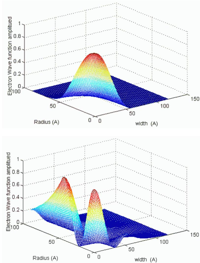
Fig. 6. (a, top) The electron ground-state wave function amplitude squared as a function of  $R$  and  $z$ . (b) The same as in (a) but of the electron first excited state.
