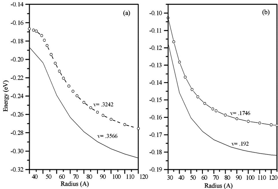
Fig. 3. (a) The electron ground-state energy as a function of radius  $R$ , for two values of the confinement potential  $V = 0.3242$  and  $0.3566$  eV, where  $L/2 = 60$  Å. (b) The same for the hole but at  $V = 0.1746$  and  $0.192$  eV, and also  $L/2 = 60$  Å.
