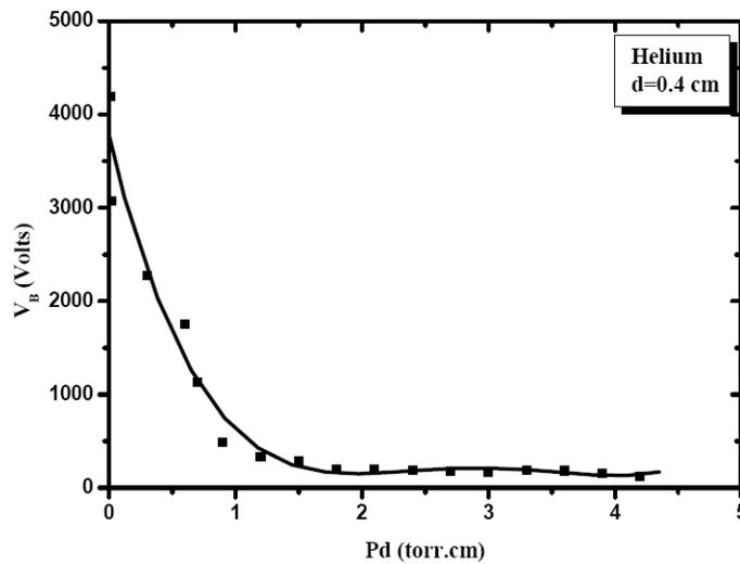
Fig. 2. Breakdown voltage  $V_B$  vs.  $Pd$  for helium discharge.
