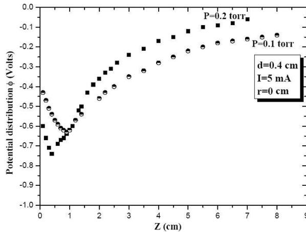
Fig. 5. Axial distribution of potential in the discharge tube.
