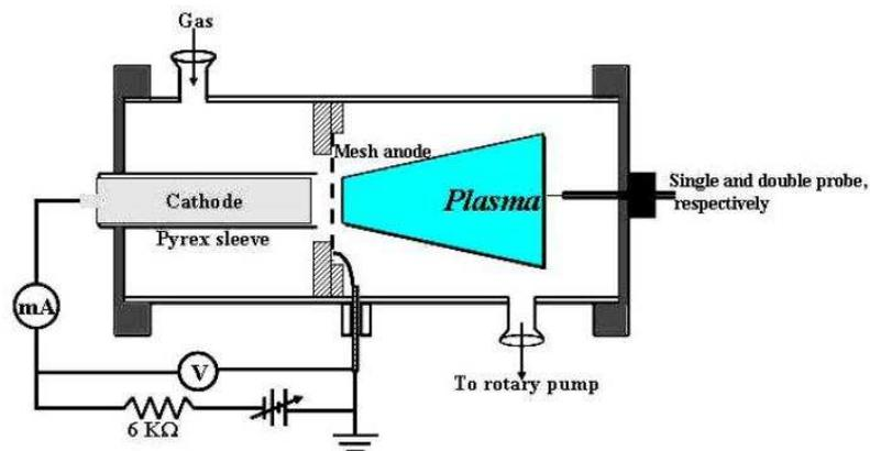
Fig. 1. Schematic diagram of the pseudo-discharge experiment.
