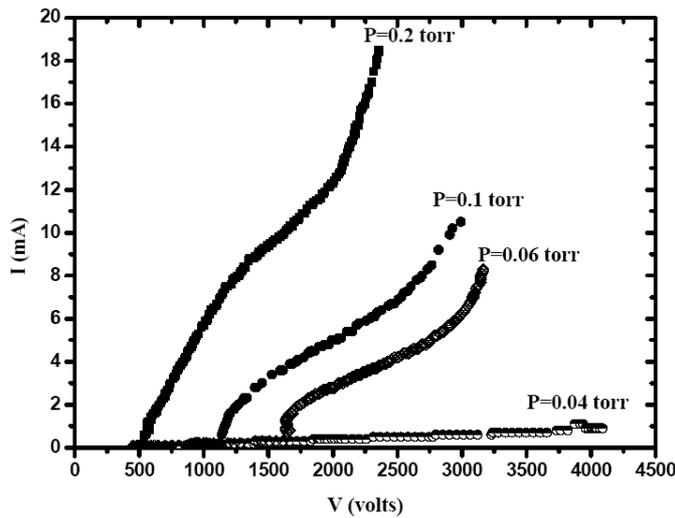
Fig. 3. Current–voltage characteristics of VC pseudo discharge.
