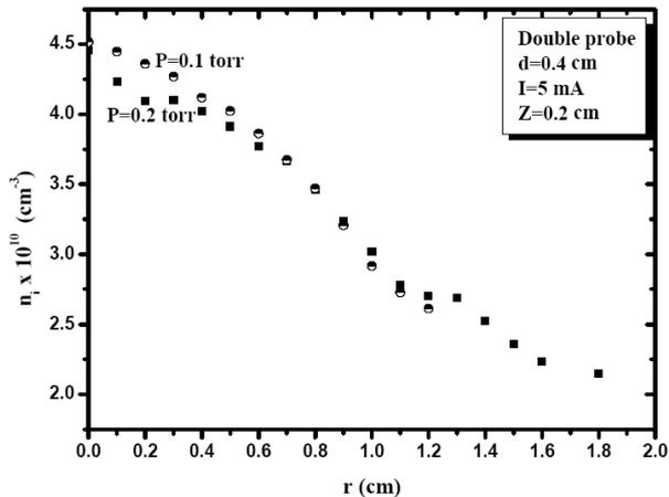
Fig. 10. Radial distribution of ion density.
