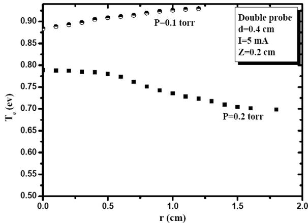
Fig. 9. Radial distribution of electron temperature.
