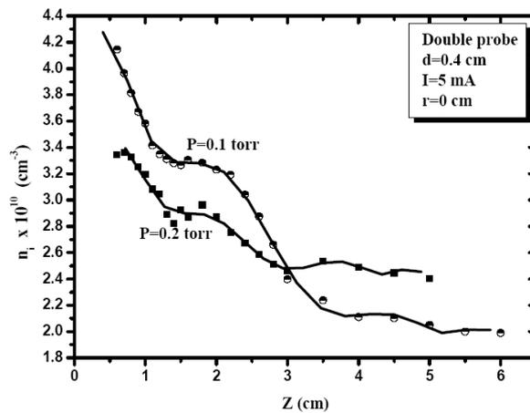
Fig. 8. Axial distribution of ion density.
