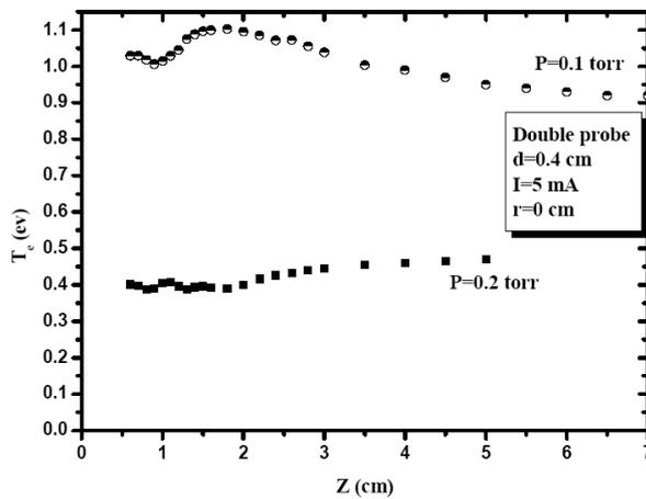
Fig. 7. Axial distribution of electron temperature.
