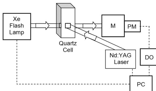
Fig. 1. Scheme of the laser flash-photolysis set-up. M - monochromator, PM - photomultiplier, DO - digital oscilloscope, PC - personal computer.
