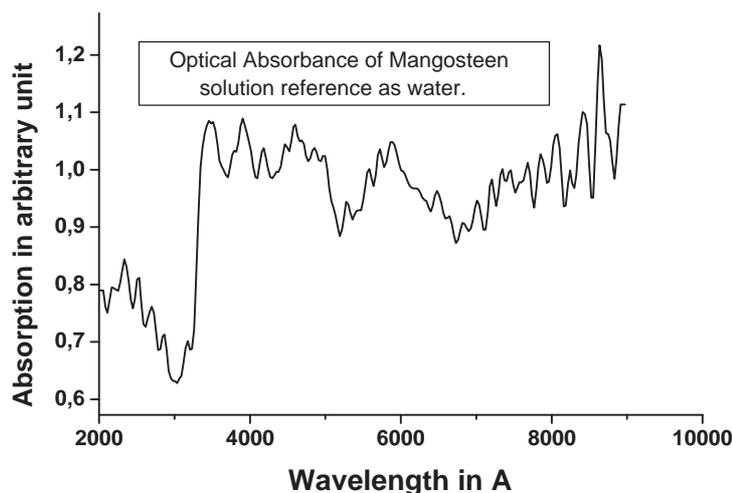
Fig. 7. UV-VIS absorption pattern of mangosteen solution in water at RT, reference water.
