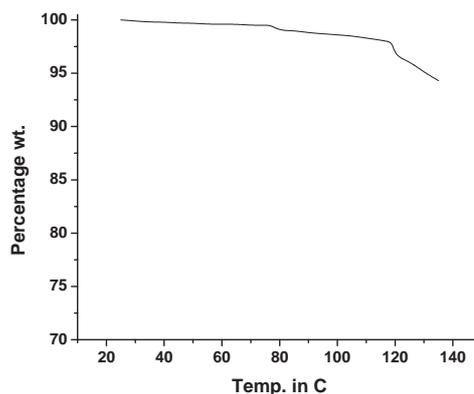
Fig. 2. Percentage loss in weight ( $w$ ) vs. temperature ( $t$ ) in deg. centigrade (Sample weight 14.0 mg). Heating rate  $5^\circ\text{C}/\text{minute}$ .
