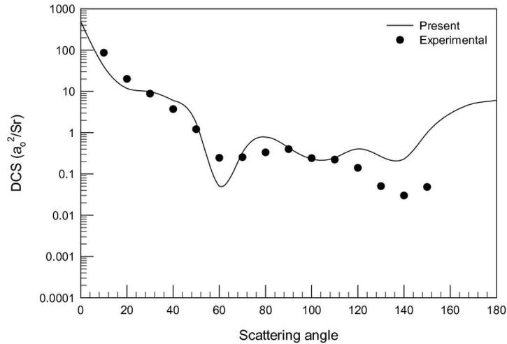
Fig. 4. Differential cross sections for electron scattering from Yb atoms at energy 60 eV.
