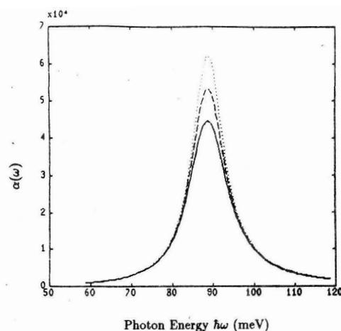
Fig. 4. Total absorption coefficient,  $\alpha(\omega)$ , versus photon energy,  $\hbar\omega$ , at  $F = 0$ . The three peaks stand for three different optical intensities: (i)  $I = 0$  (dotted line), (ii)  $I = 0.5$  MW/cm<sup>2</sup> (dashed line) and (iii)  $I = 1.0$  MW/cm<sup>2</sup> (solid line).
