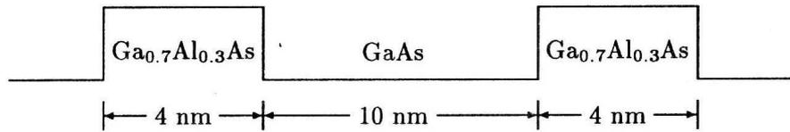
Fig. 1.  $\text{Ga}_{0.7}\text{Al}_{0.3}\text{As}$ -GaAs- $\text{Ga}_{0.7}\text{Al}_{0.3}\text{As}$  quantum well.
