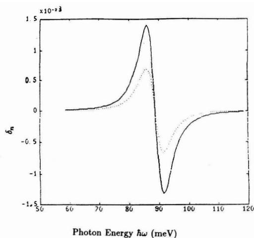
Fig. 7. The change of refractive index,  $\delta n$ , versus photon energy,  $\hbar\omega$ , with  $F = 0$  and two different values of optical intensities: (i)  $I = 0.5$  (dotted line) and (ii)  $I = 1.0$  (solid line).
