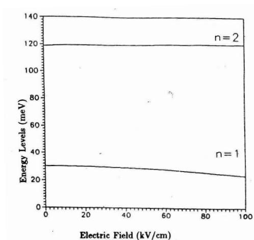
Fig. 2. The ground state ( $n = 1$ ) and the first excited state ( $n = 2$ ) energy levels, versus applied electric field.
