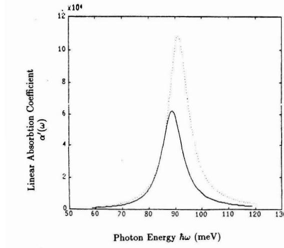
Fig. 3. Linear absorption coefficient,  $\alpha'(\omega)$ , versus photon energy,  $\hbar\omega$ , with  $F = 0$  (solid line) and  $F = 50$  kV/cm (dotted line).
