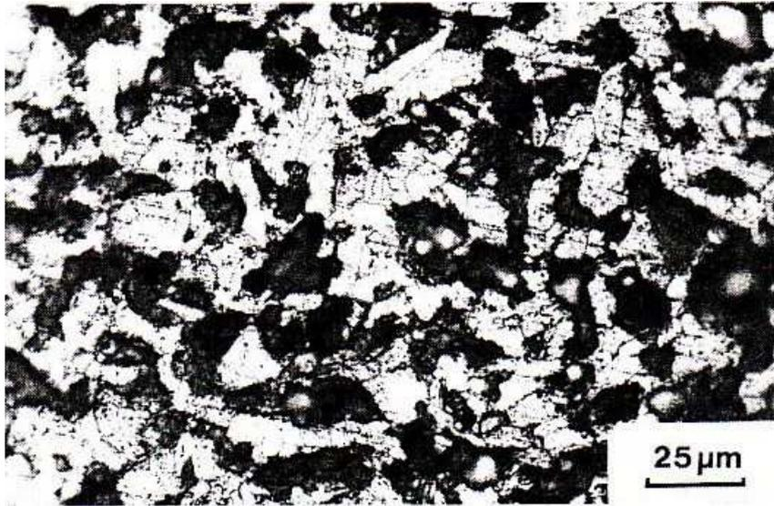
Fig. 1. Optical micrograph of the  $\text{YBa}_2\text{Cu}_3\text{O}_{7-x}$  ceramic, sample NOZ 1-I (aged for 7 hours at  $960^\circ\text{C}$ ), polished with diamond paste and etched for 5 seconds in a mild solution of HCl in distilled water.
