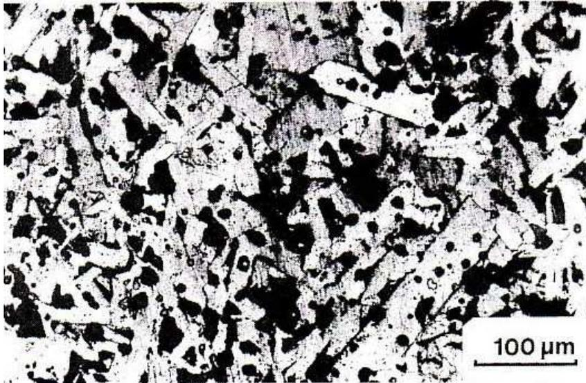
Fig. 2. Optical micrograph of the  $\text{YBa}_2\text{Cu}_3\text{O}_{7-x}$  ceramic, sample NOZ 1-II (aged for 70 hours at  $960^\circ\text{C}$ ), polished with diamond paste and etched for 5 seconds in a mild solution of HCl in distilled water.
