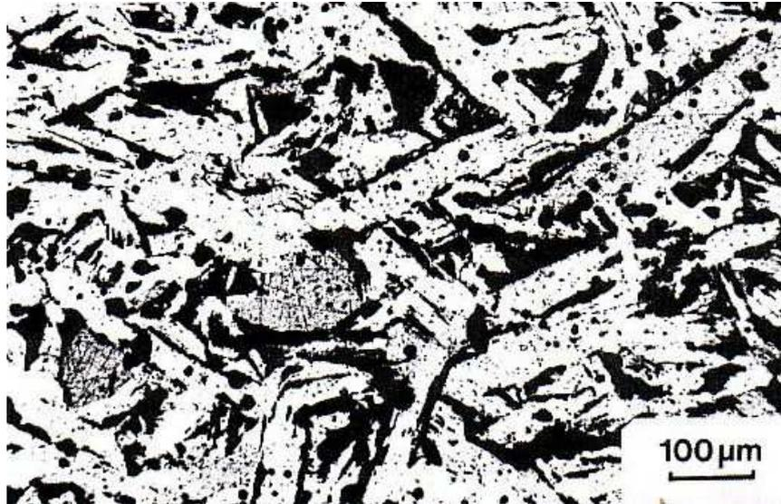
Fig. 3. Optical micrograph of the  $\text{YBa}_2\text{Cu}_3\text{O}_{7-x}$  ceramic, sample NOZ 1-III (aged for 700 hours at  $960^\circ\text{C}$ ), polished with diamond paste and etched for 5 seconds in a mild solution of HCl in distilled water.
