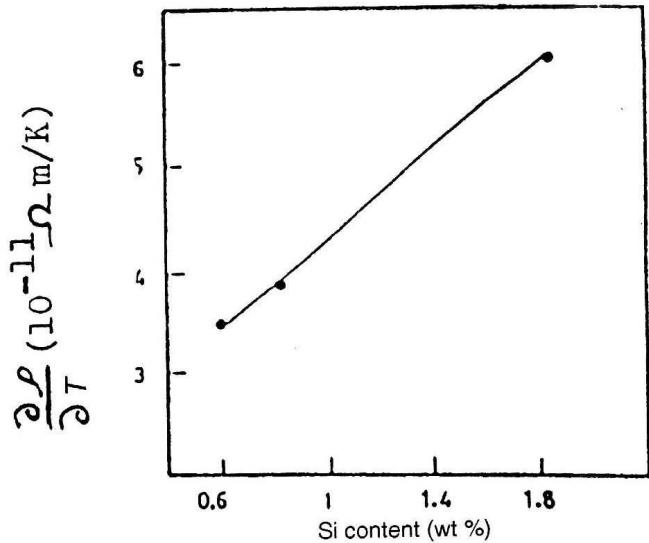
Fig. 3. Dependence of  $(\partial\rho/\partial T)$  on silicon content.
