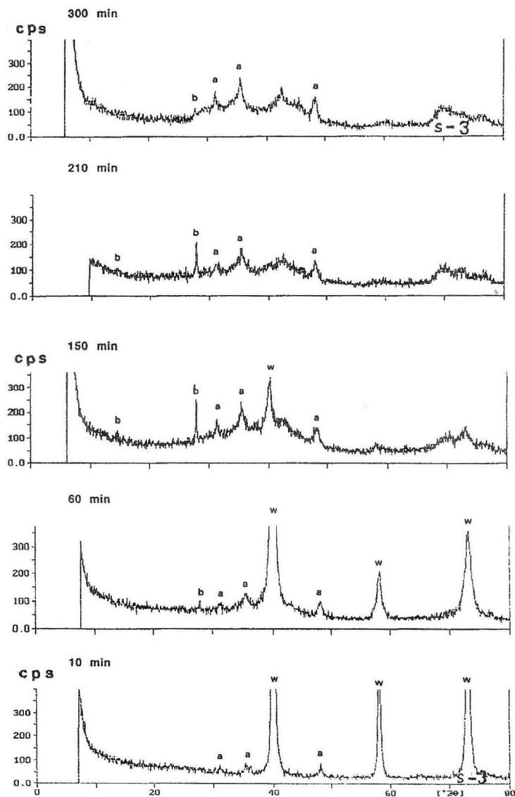
Fig. 2. Changes in the XRD pattern observed during the ball-mill processing of the powder mixture sample S-3, atomic ratio  $W:B=2:5$  in air atmosphere and at room temperature. The numbers denote milling times, and the angular positions of observed diffraction lines belonging to the WC, cubic  $B_2O_3$  and W phases that are marked with (a), (b) and (w), respectively.
