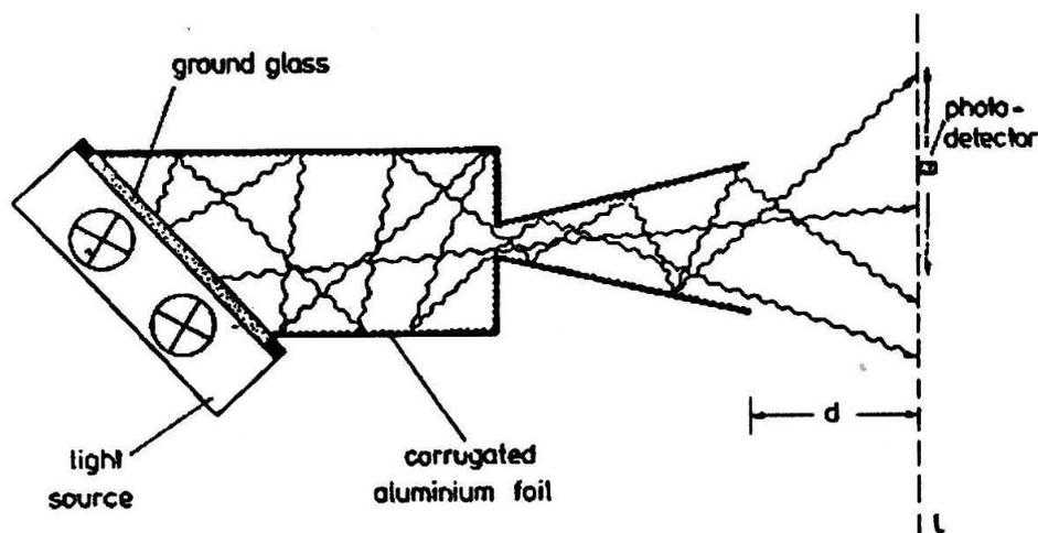
Fig. 14. Idea of light simulation of an effusive molecular beam produced in an MBE cell.
