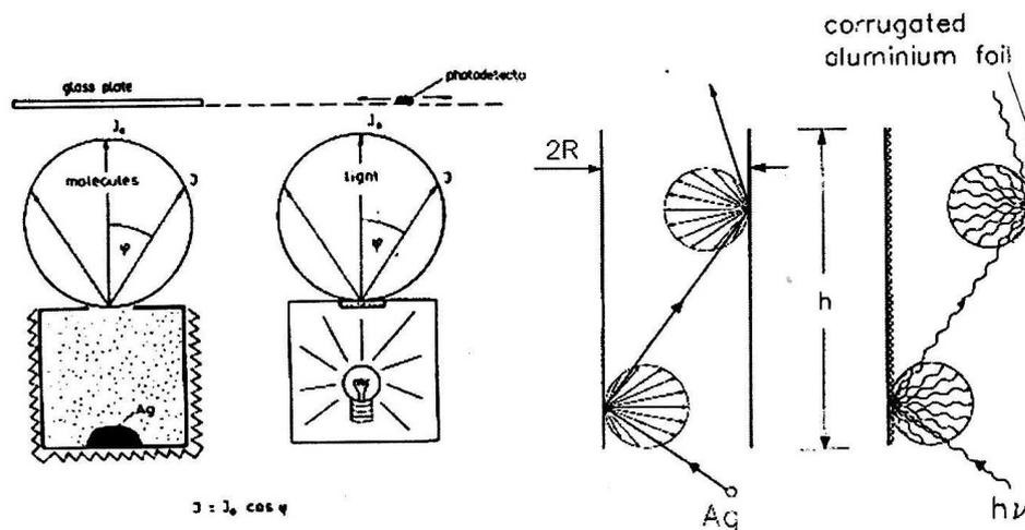
Fig. 1. Cosine-shaped intensity distribution of (a) the molecular beam formed by the round effusion hole in the Knudsen's cell, (b) the light beam formed by the round diffusion glass plate illuminated with a bulb at the back.
