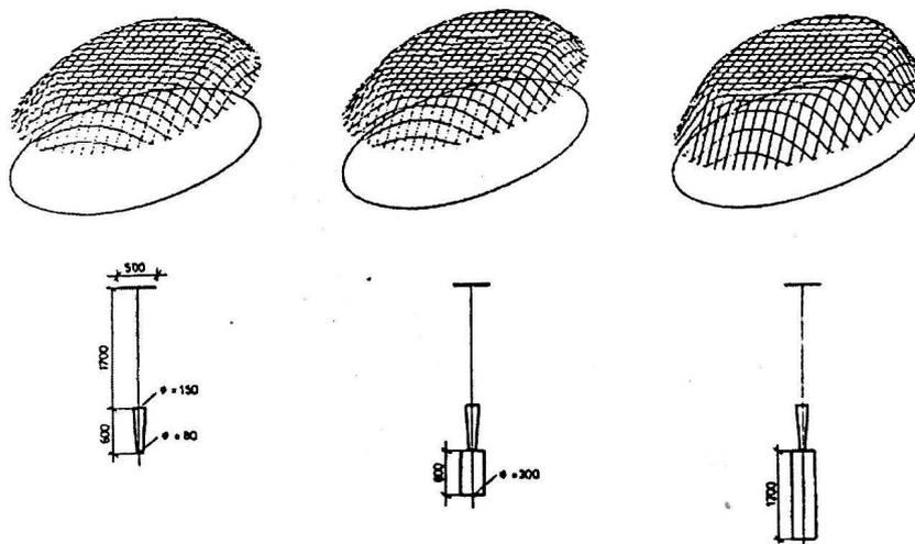
Fig. 17. Distributions of light "effusion" beams generated by three different channels as shown.
