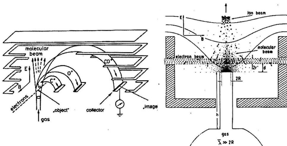
Fig. 9. Diagram of cycloidal mass spectrometer with a total ion transmission between the point of generation ( $l_0$ ) in the source and the collector.
