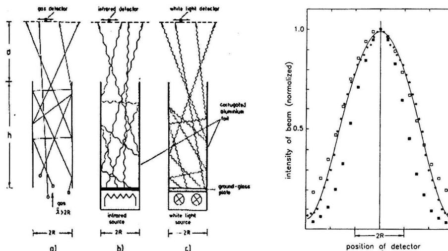
Fig. 3. (a) Effusion molecular beam formed by the effusion channel. (b) "Effusion" infrared light beam formed by the modelling tube. (c) "Effusion" white light beam formed by the modelling tube.
