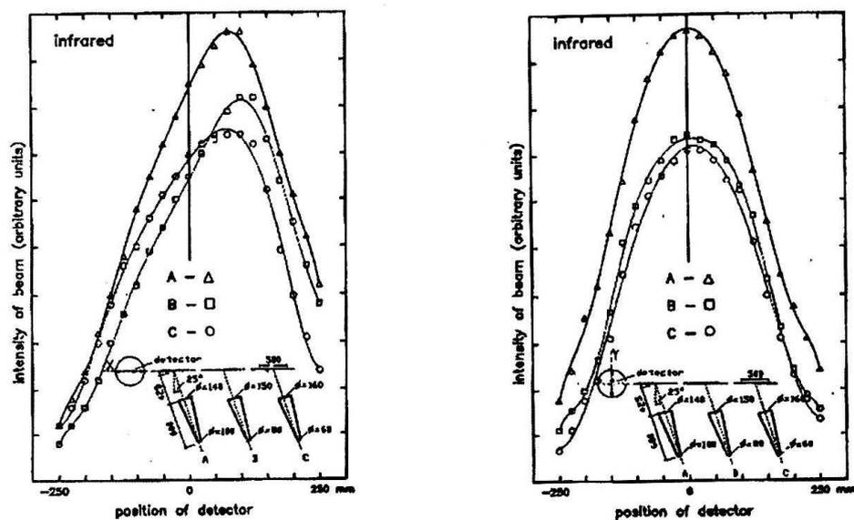
Fig. 18a. Distribution (along the X-direction) of infrared beams generated by three different channels. The plate is exposed diagonally to a beam at the angle  $25^\circ$ .
