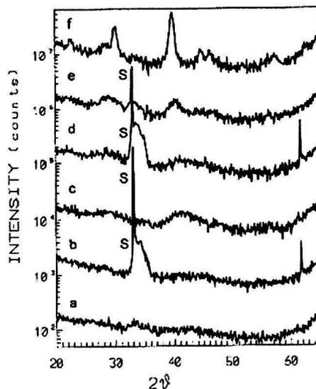
Fig. 3. LAXD spectra of W<sub>0.33</sub>Si<sub>0.66</sub>/Si ML: a – as-deposited, b – annealed at 500 °C/30 s, c – annealed at 500 °C/25 min, d – annealed at 750 °C/30 s, e – annealed at 850 °C/30 s, f – annealed at 1000 °C/30 s; S – substrate. Spectra b, c, d, e and f are multiplied by factors of 10, 10<sup>2</sup>, 10<sup>3</sup>, 10<sup>4</sup> and 10<sup>5</sup>, respectively.
