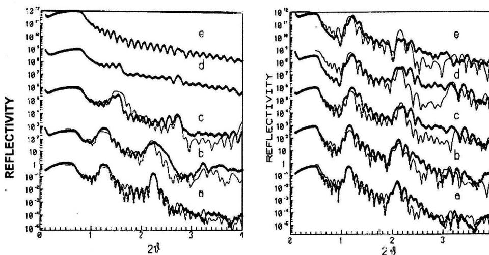
Fig. 1. X-ray reflectivity spectra of W/Si ML: a – as-deposited, b – annealed at 500 °C/30 s, c – annealed at 500 °C/25 min, d – annealed at 750 °C/30 s, e – annealed at 850 °C/30 s. Spectra b, c, d and e are multiplied by factors of  $10^3$ ,  $10^6$ ,  $10^9$  and  $10^{12}$ , respectively. The simulated spectra are shown by thin line.
