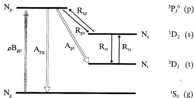
Fig. 2. Schematic diagram of the barium levels relevant for the model applied (see Section 3);  $\rho B$  – pumping rate;  $A$  – spontaneous emission rates;  $R$  – collisional mixing rates;  $N$  – population density of the particular level; indices:  $g$  – ground state,  $p$  – optically excited state,  $s$  – singlet metastable state,  $t$  – triplet metastable state.
