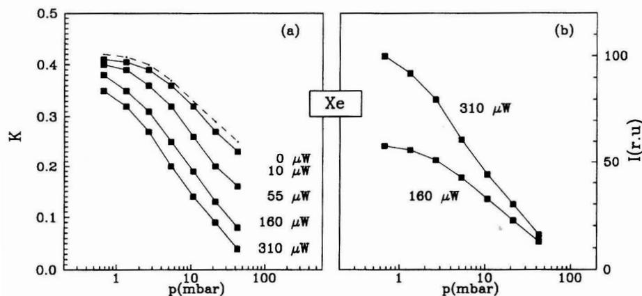
Fig. 4. (a) Plot of the optical depths  $K = k_{791.3}^0 L$  of the barium 791.3 nm line vs. xenon pressure in dependence on the laser beam power. The dashed line represents the extrapolation to zero power (1 bar =  $10^5$  Pa). (b) The relative fluorescence intensity of the barium 791.3 nm line as a function of the xenon pressure, obtained for the two different pumping powers.
