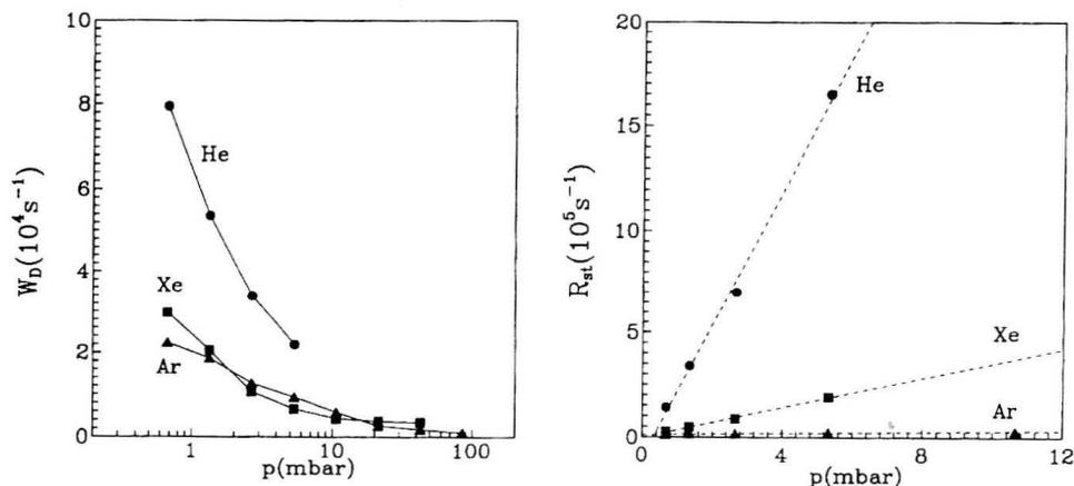
Fig. 5. Plot of the diffusion removal rate  $W_D$  versus the noble gas (He, Ar or Xe) pressure.
