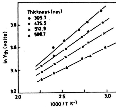
Fig. 7. Variation of threshold voltage  $V_{th}$  with temperature for  $ZnIn_2Se_4$  thin films of different thickness.
