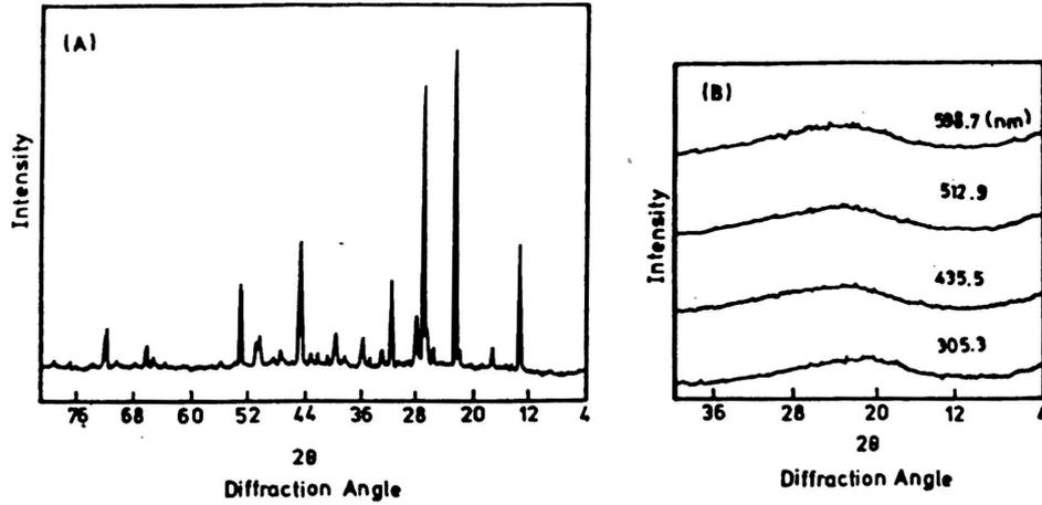
Fig. 1. X-ray diffraction pattern (A) powder form, (B) thin films.
