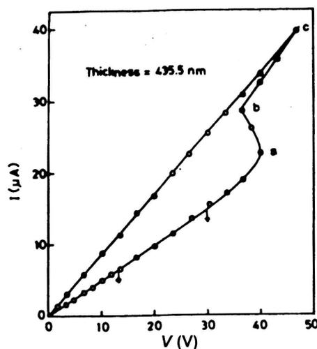
Fig. 3. Static  $I - V$  characteristic curve for  $\text{ZnIn}_2\text{Se}_4$  thin film of thickness 435.5 nm.
