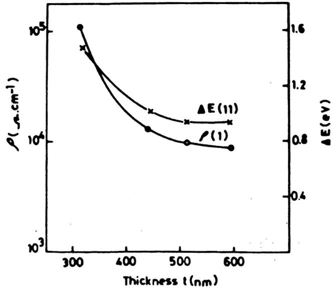
Fig. 2. Variation of  $\rho$  and  $\Delta E$  with film thickness.
