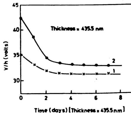
Fig. 4. Variation of threshold voltage,  $V_{th}$ , with aging period for  $ZnIn_2Se_4$  thin film: curve 1 after annealing, curve 2 before annealing.
