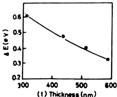
Fig. 8. Variation of the threshold voltage activation energy  $\Delta E$  with the film thickness.
