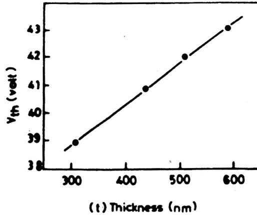
Fig. 6. The dependence of the mean value of the threshold voltage,  $V_{th}$ , on the sample thickness ( $t$ ).
