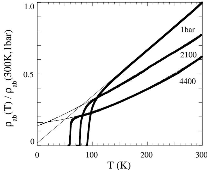
Fig. 3. Normalized resistivity measured in the  $ab$  plane of  $\text{Bi}_2\text{Sr}_2\text{CaCu}_2\text{O}_{8-y}$  overdoped at high oxygen pressure (marked in bars at the annealing temperature of  $450^\circ\text{C}$ ). The 4400 and 1 bar curves correspond to the same crystal.
