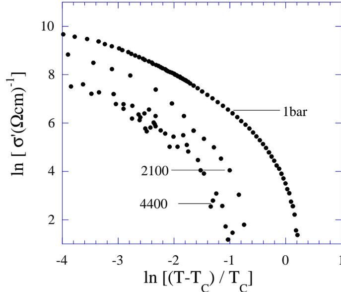
Fig. 4. Fluctuation analysis of data in Fig. 3. The excess conductivity was extracted by the extrapolation of the  $T_m$  superlinear behaviour of the temperature dependence of the resistivity of the overdoped samples ( $m = 1.16$  and  $1.65$  for the 2100 and 4400 samples, respectively).
