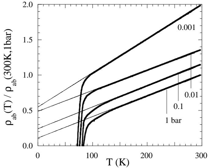
Fig. 1. Normalized resistivity measured in the  $ab$  plane for the same single crystal of  $\text{Bi}_2\text{Sr}_2\text{CaCu}_2\text{O}_{8-y}$  at various oxygen contents  $y$ . The numbers on the curve refer to the oxygen partial pressure (in bars) at the annealing temperature [14].
