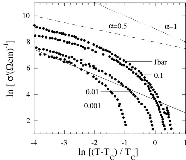
Fig. 2. Fluctuation analysis of data in Fig. 1,  $\sigma'$  is the excess conductivity. The dashed lines show the slopes expected ( $-0.5$  and  $-1$ ) in the 3D and 2D limits of Eq. (1). The straight solid line shows the 2D limit of Eq. (1) using  $S = 1.5$  nm and a room temperature resistivity of  $150 \mu\Omega\text{cm}$ .
