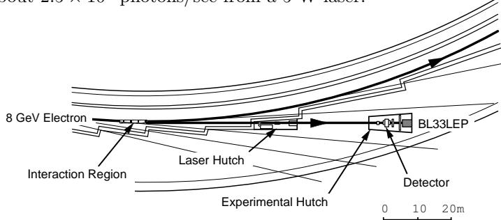
Fig. 1. The laser electron photon beamline at SPring-8.
