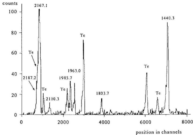
Fig. 1. Spectrum of the reaction  $^{133}\text{Cs}(d, ^3\text{He})^{132}\text{Xe}$ . The lines of  $^{132}\text{Xe}$  are labelled with their energy in keV (values from current NDS) while the lines of  $^{126}\text{Te}$  are simply labelled with 'Te'. The energy of the incident deuterons was 27 MeV and the angle of observation was  $30^\circ$  in the laboratory system. The resolution was about 7.5 keV FWHM. Furthermore the remarkable low background should be mentioned.
