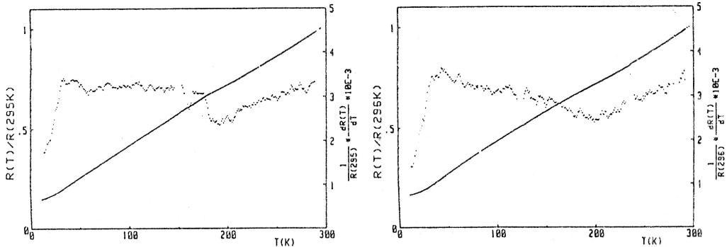
Fig. 2 Resistivity and its temperature derivative of  $\text{NbTe}_4$ , of "good quality" (a) and of "poor" one (b).
