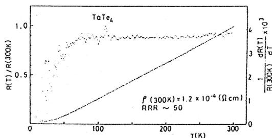
Fig.1 Resistivity along the c-axis and its temperature derivative of TaTe<sub>4</sub>
