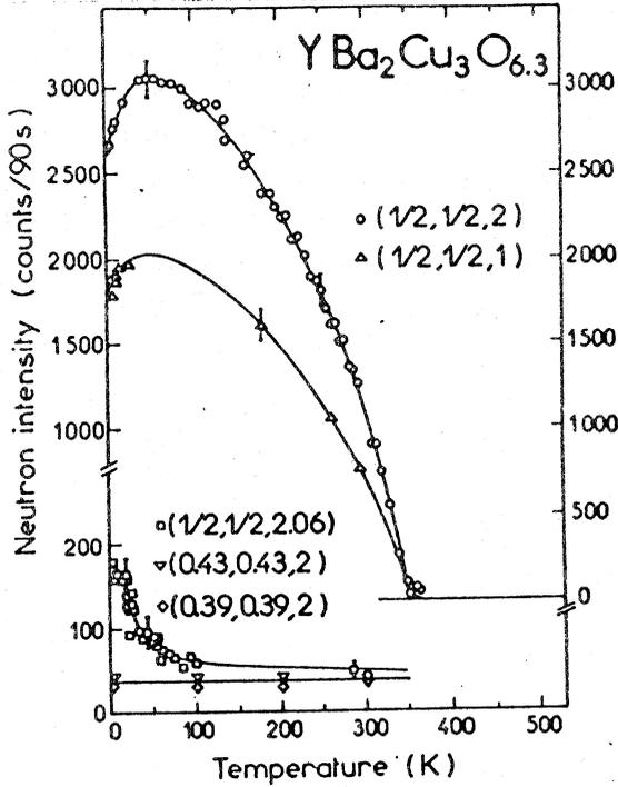
Fig.2 Temperature dependence of the magnetic Bragg intensity and of the diffuse scattering for YBa<sub>2</sub>Cu<sub>3</sub>O<sub>6+x</sub> with x=0.3 and 0.37.
