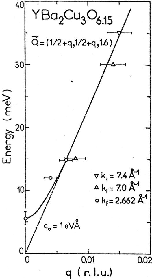
Fig.5 Spin wave energies for small wave vectors around the antiferromagnetic Bragg point of the AF sample YBa<sub>2</sub>Cu<sub>3</sub>O<sub>6.15</sub>. The dotted line corresponds to a spin wave velocity  $c_0 = 1 \text{ eV \AA}$ .
