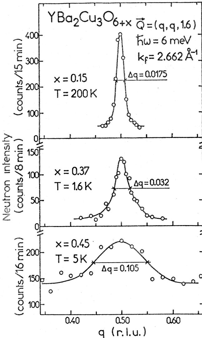
Fig.4 Q-scans performed for an energy transfer  $\hbar\omega=6$  meV for  $\text{YBa}_2\text{Cu}_3\text{O}_{6+x}$  with  $x=0.15, 0.37, 0.45$ . The  $q$ -width due to the resolution is  $\Delta=0.017$  r.l.u.
