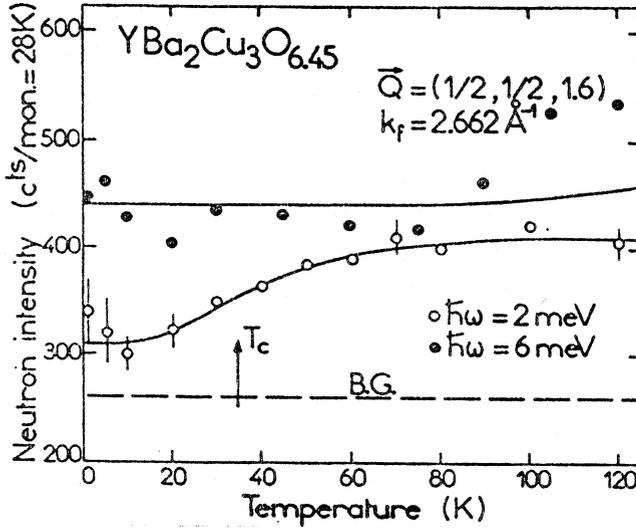
Fig.7 Magnetic intensity as a function of temperature measured at  $\vec{Q} = (1/2, 1/2, 1.6)$  for energy transfers  $\hbar\omega = 2$  and 6 meV for YBa<sub>2</sub>Cu<sub>3</sub>O<sub>6.45</sub>
