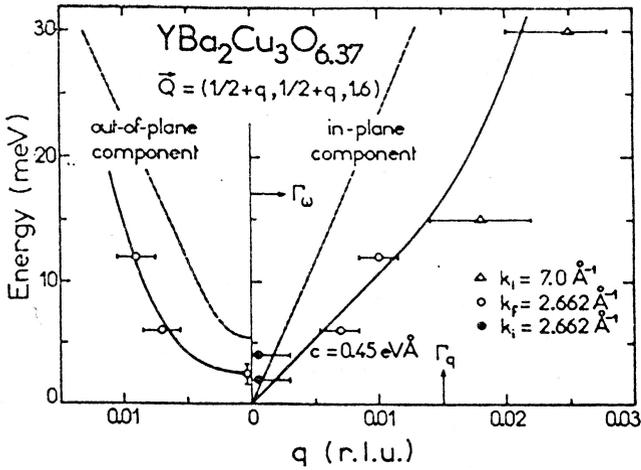
Fig.6 Excitation energies of in-plane and out-of-plane spin components for  $\text{YBa}_2\text{Cu}_3\text{O}_{6.37}$ . The renormalization of excitation energies is large at small  $q$  as shown by the comparison with the undoped sample (dotted line).
